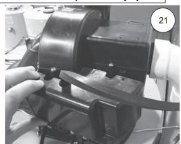
Remove Three screws (Phillips Screw driver) from control access cover on blower and remove cover (see photo 21).
