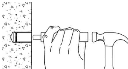
Using the tool, set the anchor by driving the lead sleeve over the cone using several sharp hammer blows. Be sure the anchor is at the required embedment depth so that anchor threads do not protrude above the surface of the base material. Position the fixture, insert screw or bolt and tighten.
