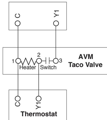
Figure 21: Taco SBV Valve Wiring
