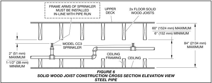
depth is 6 in. (152 mm) from the bottom of the upper chord to the top of the lower chord.
