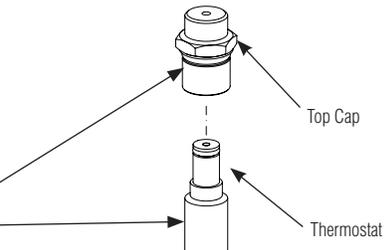
**B** Insert a 7/16" dia. rod into the valve until it touches the top of the pushrod that is attached to the piston. Mark the length of the rod inside the valve. Push the rod until the piston stops and mark the new length.
