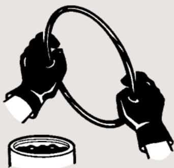
Lubricate the gasket thoroughly before it is placed on the spigot or tongue.
