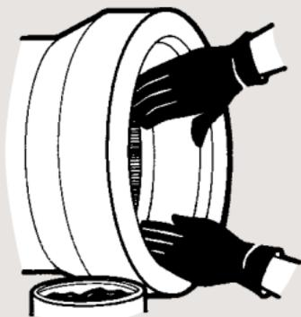
Lubricate bell jointing surface liberally. Use a brush, cloth, sponge or gloves to cover entire surface. Only approved lubricant should be used.
