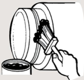
Lubricate the spigot or tongue end of pipe, especially the gasket recess.
