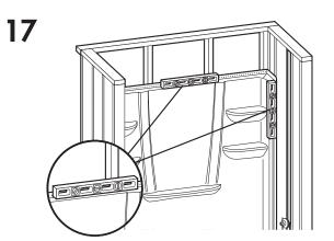
Level back wall vertically & horizontally. Shim if necessary.
