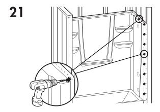
Fasten flanges along top of right side wall with fasteners of choice (see Pre-Installation Planning #12) into each corresponding stud. Fasten side (vertical) flanges to side studs 8" (200mm) on center.
