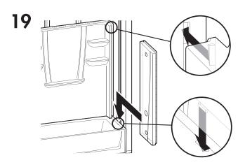
Slide right side wall into position. Be sure locking mechanism is engaged. **NOTE:** Caulking is not required, however, if using caulk, weep channel must remain clear of obstruction to allow for proper drainage of the unit.
