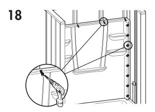
Fasten flanges along top of back wall with fasteners of choice (see Pre-Installation Planning #12) into each corresponding stud. Pre-drill both (vertical) side flanges and nail fasten to side studs 8" (200mm) on center. **NOTE:** A stud should be added if adding accessories. Must have at least 1 fire block to secure vertically.
