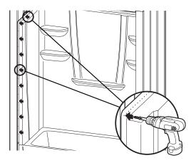
Fasten flanges along top of left side wall with fasteners of choice (see Pre-Installation Planning #12) into each corresponding stud. Fasten side (vertical) flanges to side studs 8" (200mm) on center.
