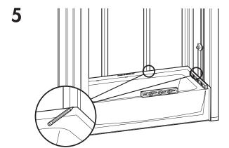
Level and mark all sides. Front apron should be firmly on the floor.
