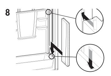
Slide right side wall into position. Be sure locking mechanism is engaged.
