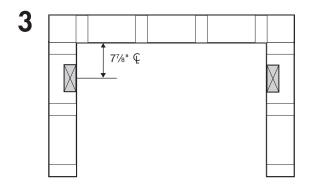
Pre-install unit to ensure framing pocket is plumb, square and a level installation can be achieved (see steps 3 through 9).
