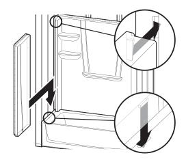
Slide left side wall into position. Be sure locking mechanism is engaged. NOTE: Caulking is not required, however, if using caulk, weep channel must remain clear of obstruction to allow for proper drainage of the unit.
