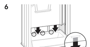
Lift and place the back wall, making sure locking tabs are engaged.
