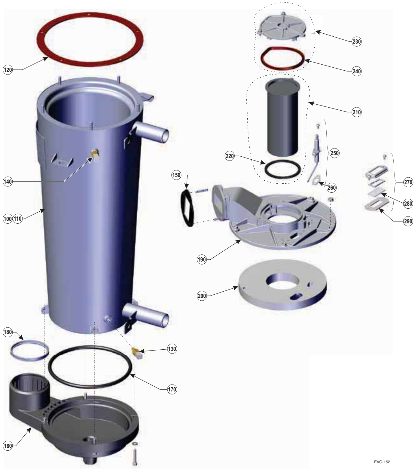
Figure 117 Heat exchanger assembly EVG 155 (see Figure 116, page 132 for part numbers)
