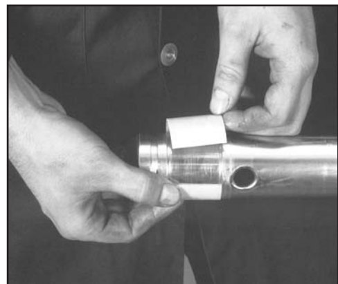
FIG. 73: POSITION REAR SLIDE TAPE
