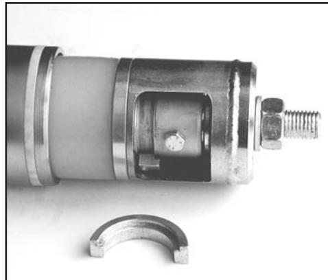
FIG. 62: REMOVE SEGMENTED RINGS
