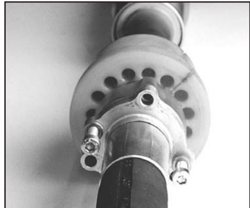
FIG. 58: 2 SCREWS USED AS JACK SCREWS
