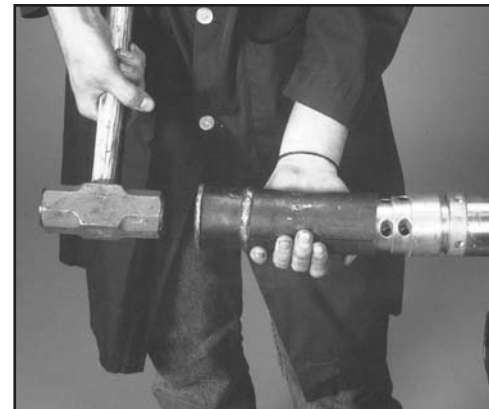
FIG. 31: USING PIPE TO SECURE STEPPED CONE
