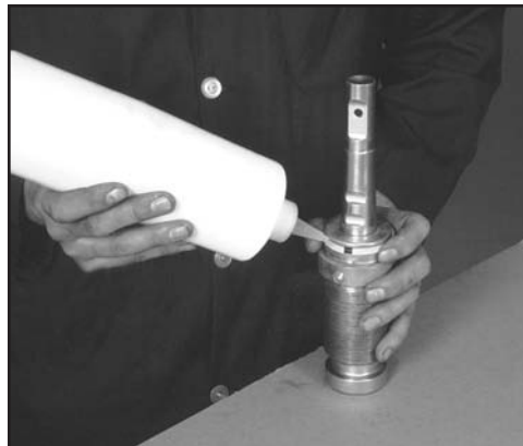
FIG. 30: GREASE THE SEAL
