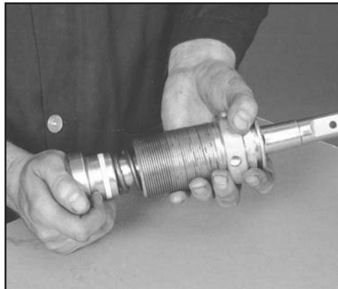
FIG. 27: INSERT THE CHISEL
