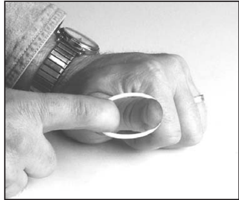
FIG. 46: STRETCH NEW SEAL TO FIT CONTROL STUD
