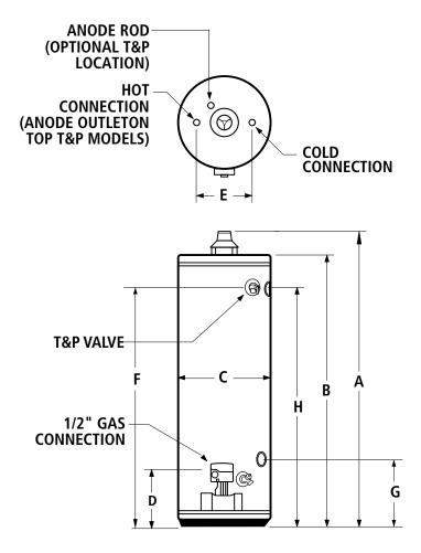
**Maximum Hydrostatic Working Pressure: 150 PSI**
