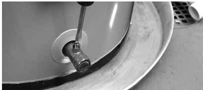
Figure 42 - Draining the water heater.
