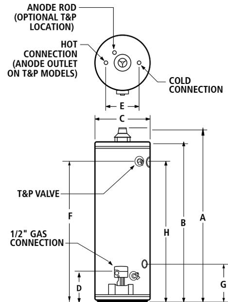
Maximum Hydrostatic Working Pressure: 150 PSI
