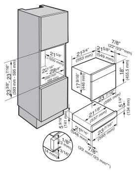
② Installation dimensions with plug Power cord L= 7' 2 5/8" (2200 mm)
