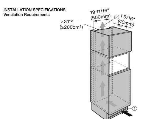
Air intake  $\ \, \mathbb O \$  occurs via the plinth at the bottom of the appliance and the air escapes at the top  $\ \, \mathbb O \$  at the rear of the surrounding cabinets.
