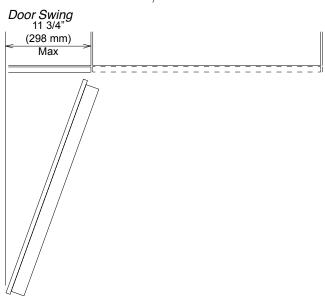
**NOTE**: Additional space needed depending on the thickness of front panels and handle used.
