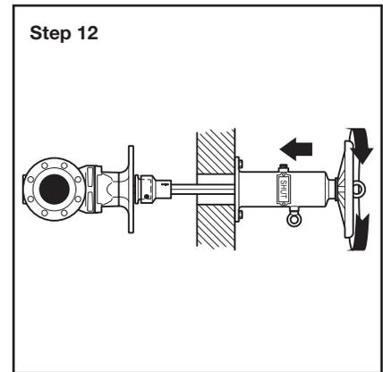
**Step 12.** Rotate Handwheel counter-clockwise until SHUT Targets are centered in Cap windows. Ensure that Gate Valve is fully shut.
