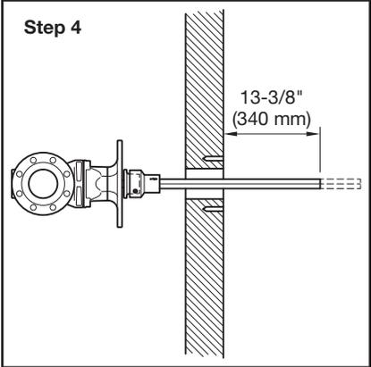
**Step 4.** Mark Extension Rod 13-3/8 inches (340 mm) from wall. Remove Extension Rod Assembly and evenly cut extension Rod at marked location.
