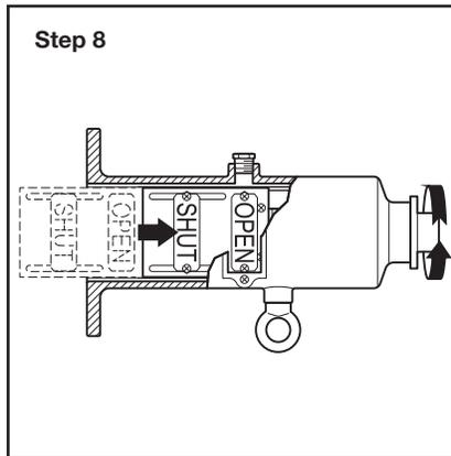
**Step 8.** Position Target Carrier in Cap cavity and engage Operating Stem by Stem Nut. Rotate Operating Stem clockwise until OPEN Targets are centered in Cap windows.
