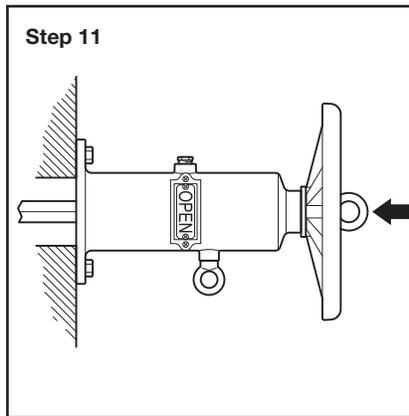
**Step 11.** Attach Handwheel to Cap Assembly and secure with Eyebolt and Washer.
