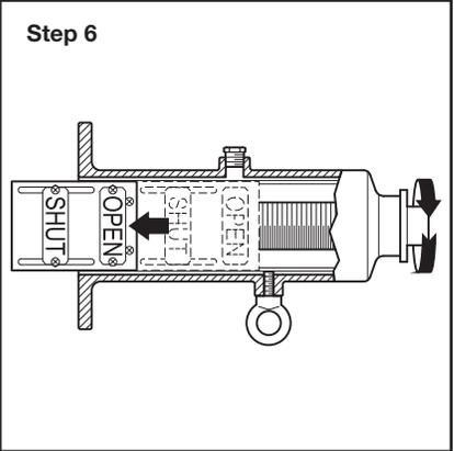
**Step 6.** Rotate Operating Stem counterclockwise to remove Target Carrier from Cap.
