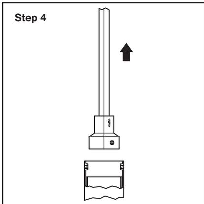
**Step 4.** Remove Extension Rod from Post Assembly.
