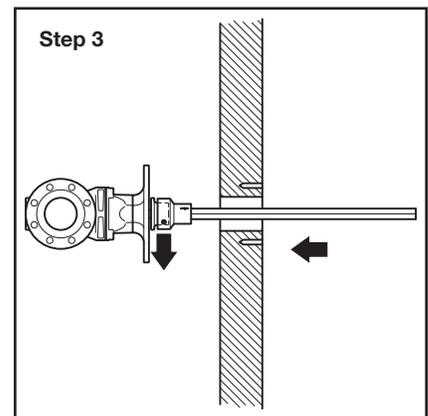
**Step 3.** Loosen Connect Cap Set Screws. Insert Extension Rod Assembly through wall clearance hole and temporarily engage Gate Valve Top Cap by Connect Cap.
