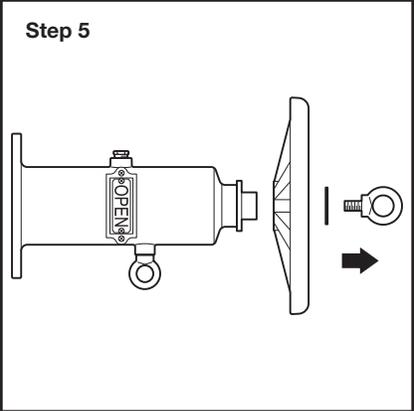
**Step 5.** Remove Eyebolt, Washer and Handwheel from Cap Assembly.
