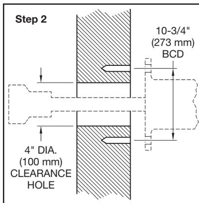
**Step 2.** Cut hole in wall for Connect Cap clearance. Drill four anchor bolt holes on 10-3/4 inch (273 mm) BCD for securing Post Body to wall in orientation shown in Step 10.
