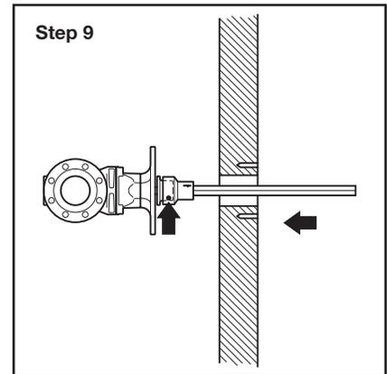
**Step 9.** Install Extension Rod Assembly engaging Gate Valve Top Cap by Connect Cap. Tighten Connect Cap Set Screws to secure.
