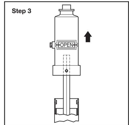
**Step 3.** Remove Cap Assembly from Post Assembly.
