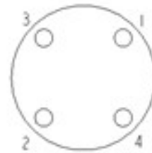
Figure 2: Bolt Tightening Sequence
