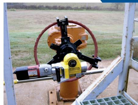
P-2 Handheld Valve Operator shown with handwheel adapter accessory
