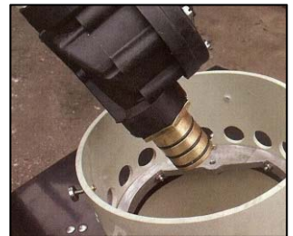
Entire valve assembly slides out!
