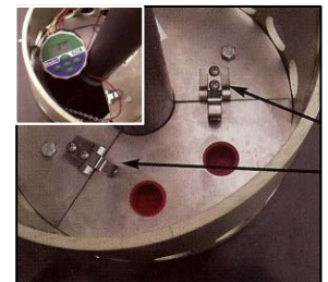
To access controller, flip thumb clips up and remove small plate
