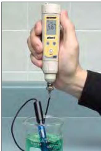
Use with direct connect or cabled electrodes.
