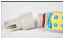
Sensor includes both pH and conductivity/TDS/salt probes.
