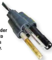
Multiprobe holder makes it easy to manage probes simultaneously.
