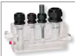
Use multiprobe flow block 35434-90 for groundwater sampling. Holds two 12-mm diameter pH, ORP, or ISE probes, one Oakton conductivity/TDS probe, and one Oakton dissolved oxygen probe.
