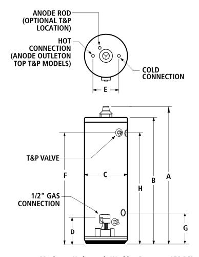
**Maximum Hydrostatic Working Pressure: 150 PSI**
