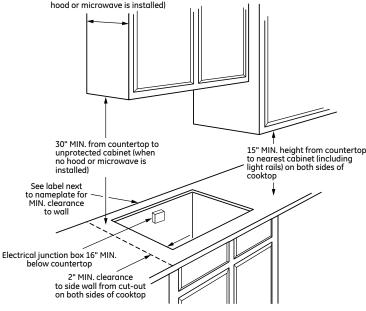
13" MAX. depth of unprotected overhead cabinets (when no
