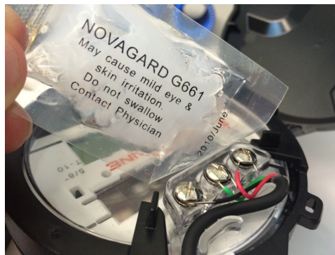
Figure 11 – Apply the Sealant
