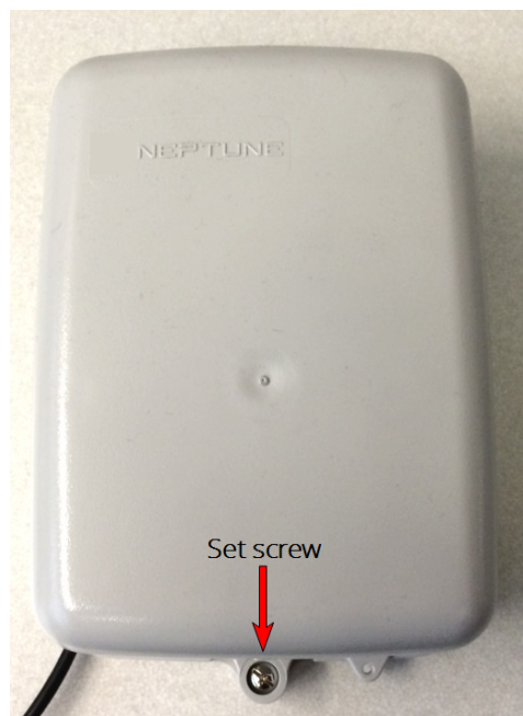
Figure 13 – Wall MIU Main Housing
