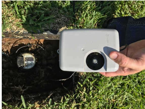
Figure 26 – MIU Housing and Latch Plate
