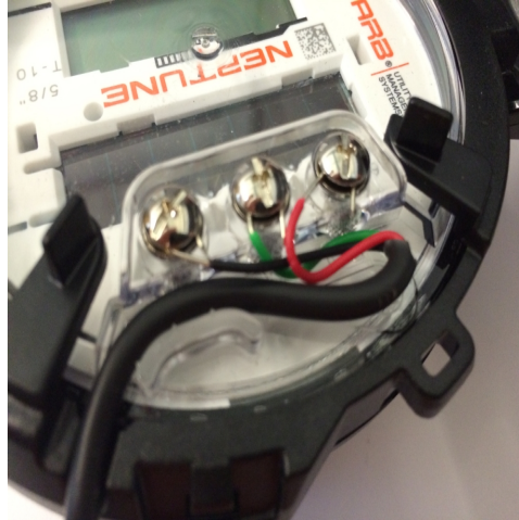
Figure 10 – Cable Threaded around Strain Relief Posts
