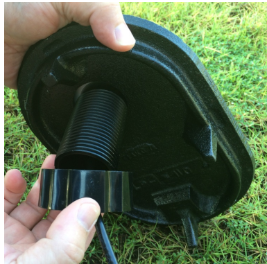
Figure 23 – Locking Nut on Antenna
