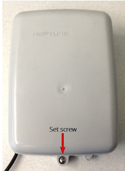
Figure 17 – Securing the Mounting Adapter
