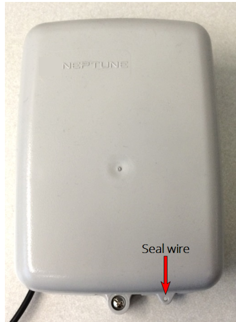
Figure 19 – Install Seal Wire
