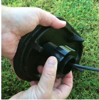
Figure 24 – Securing the Locking Nut
