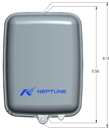
Figure 6 – Wall MIU Dimensions - Front
