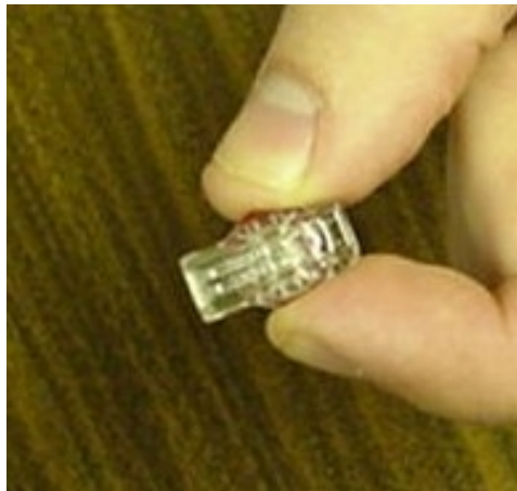
Figure 28 – 3M Scotchlok™ Connector
