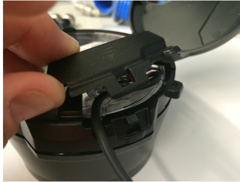
Figure 12 – Covering the Terminal Screws
