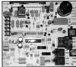
INTEGRATED FURNACE CONTROL
