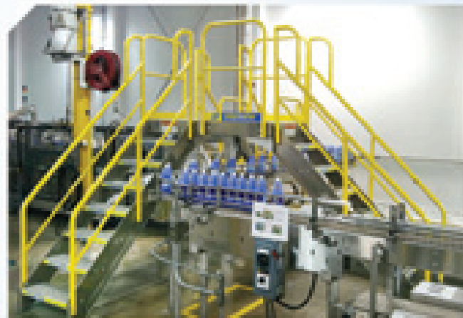
Complex crossover with multiple access points.
