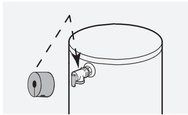
Typical Side Connect T & P Arrangement.
