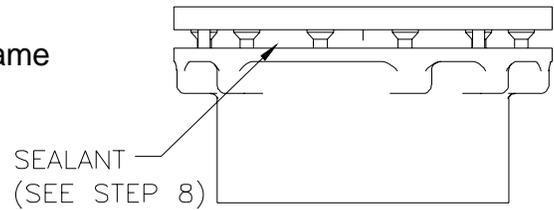
**Step 8** Apply a suitable and sufficient amount of sealant between the raised frame (D) and the cast iron head (F) to make a watertight seal.
