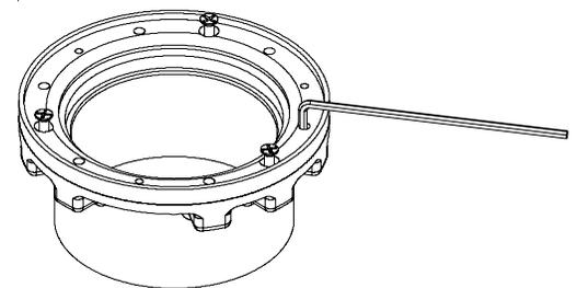
**Step 5** Turn the allen wrench counter-clockwise to loosen and raise the leveling screw (E) underneath the frame. (D)
