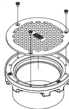
**Step 3** Loosen but do not remove the three #8-32 x 3/4 flat head screws that secure the frame (D) to the head. (F)
