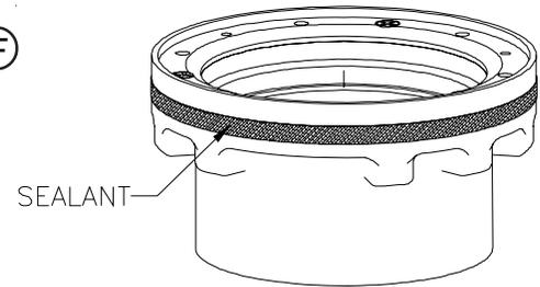
**Step 9** Replace the strainer (B) onto the frame (D) and secure strainer with the three #8-32 x 1/4 flat head strainer screws. (A)
