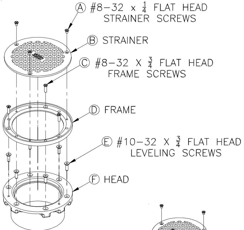
**Step 1** Loosen and remove the three #8-32 x 1/4 flat head strainer screws (A) that secure the strainer (B) to the frame. (D)
