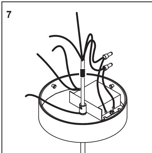
Prepare four field wires from two electrical feeds. Use a four wire cable with ground. This wiring is for operating the fixture on two separate switches. A field ground wire is necessary.
