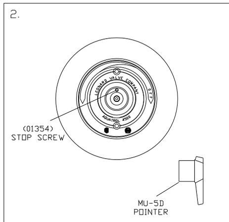
1. Remove pointer (MU-5D). Loosen 1354 stop screw, until it is flush with cover.
