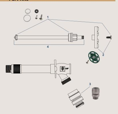
**Warning:** Frost-Proof Wall Hydrants must be installed with a downward tilt toward hose thread outlet AND the hose or other devices must be removed in cold and freezing weather. Failure to properly winterize a frost-proof wall hydrant can result in damage caused by freezing water and is not covered by under warranty.
