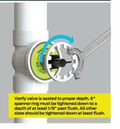
3 Turn the stem to the closed position, turning clockwise until tight. Perform test.\*\*\*
