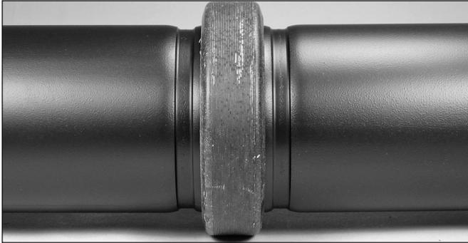
**5. JOIN PIPE/MATING COMPONENTS:** Align the two grooved ends of the pipe/mating components. Insert the other pipe/mating component end into the gasket until it contacts the center leg of the gasket. **NOTE:** Make sure no portion of the gasket extends into the groove of either pipe/mating component.
