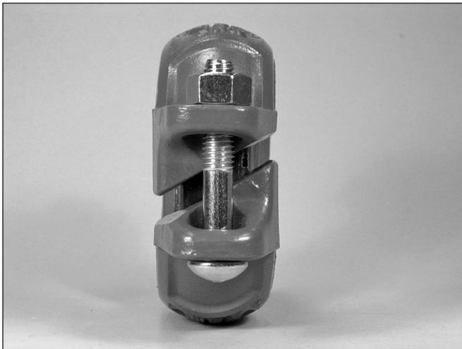
**1. DO NOT DISASSEMBLE THE COUPLING:** Style 107H/107N Couplings are installation ready. These couplings are designed so that the installer does not need to remove the bolts and nuts for installation. This design facilitates installation by allowing the installer to directly install the grooved end of pipe/mating components into the coupling.
