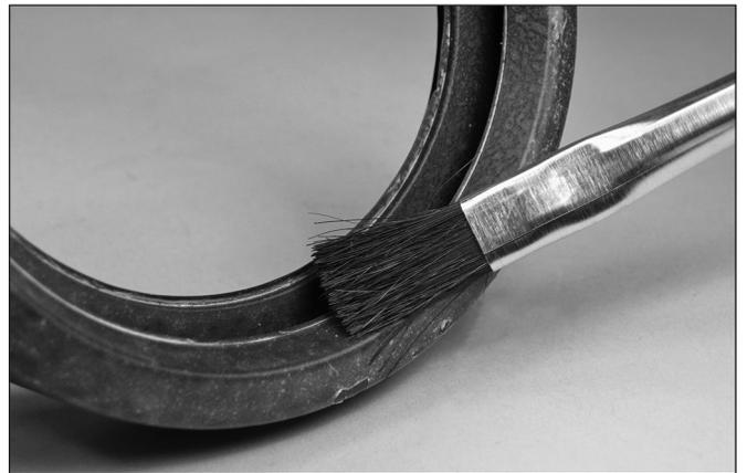
**3. FOR RE-INSTALLATION OF STYLE 107H/107N COUPLINGS, LUBRICATE GASKET:** Apply a thin coat of Victaulic Lubricant or silicone lubricant to the gasket sealing lips and exterior. It is normal for the gasket surface to have a hazy white appearance after it has been in service.
