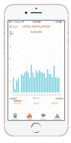
Download Intellihot's new mobile app, telli**Zero**, and start monitoring your unit. Check water inlet/outlet temperatures, flow rates, flue gas temperatures, combustion rates, and more, available on your mobile device of choice.
