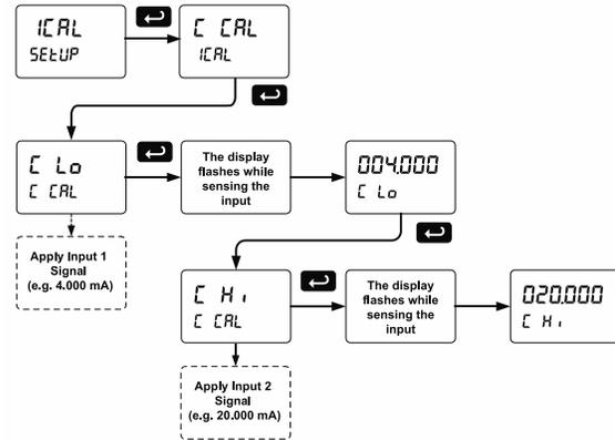
The graphic shows the calibration of the current input. The voltage input is calibrated in a similar way.
