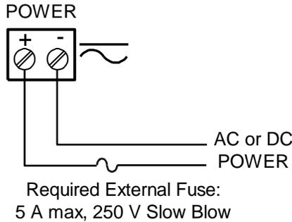
Figure 11. Power Connections
