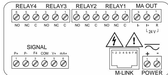
Figure 10. PD6200-##7 Connectors Label
