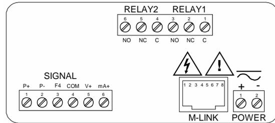
Figure 6. PD6200-##2 Connectors Label
