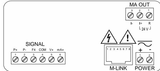
Figure 7. PD6200-##3 Connectors Label
