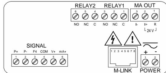
Figure 9. PD6200-##5 Connectors Label
