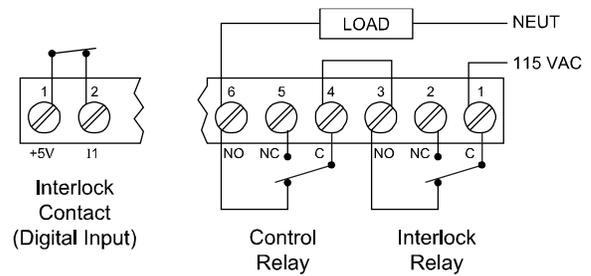
Figure 25. Interlock Connection
