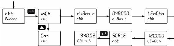
*Note: After Scale is displayed continue pressing the Enter button until the meter completes the scaling of the input and display values.*
