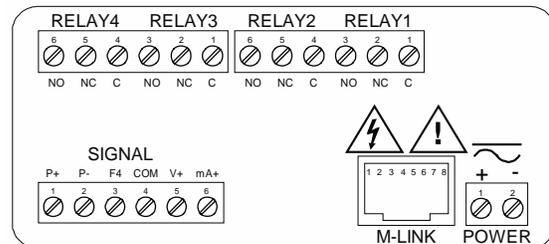
Figure 8. PD6200-##4 Connectors Label
