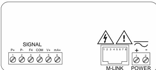
Figure 5. PD6200-##0 Connectors Label
