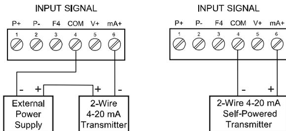
Figure 13. Transmitter Powered by External Supply or Self-Powered
