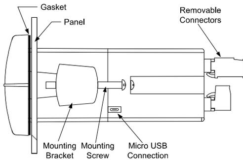
**DO NOT** apply AC or DC power to the meter when using the USB connection.
