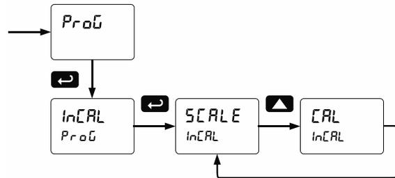
*Note: The Scale and Calibrate functions are exclusive of each other. The meter uses the last function programmed. Only one of these methods can be employed at a time. The Scale and Calibrate functions can use up to 32 points (default is 2). The number of points should be set in the Advanced menu prior to scaling and calibration of the meter. See Multi-Point Linearization (LnERr) on page 41 for details.*
