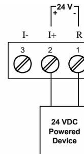
Figure 20. Analog Output Supply Powering Other Devices
