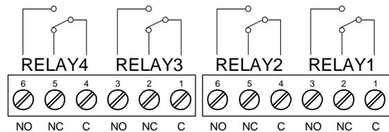
Figure 15. Relay Connections
