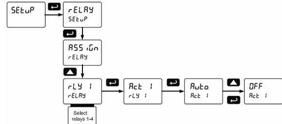
2. In the *Advanced features – User* menu program any of the digital inputs to *Force On* any of the internal relays (1-4).
