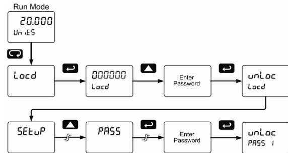
If the correct six-digit password is entered, the meter displays the message *unLoc* (unlocked) and the protection is disabled until a new password is programmed.
