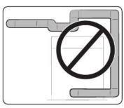
**3.** Using unnecessarily long ducts that have many elbows.
