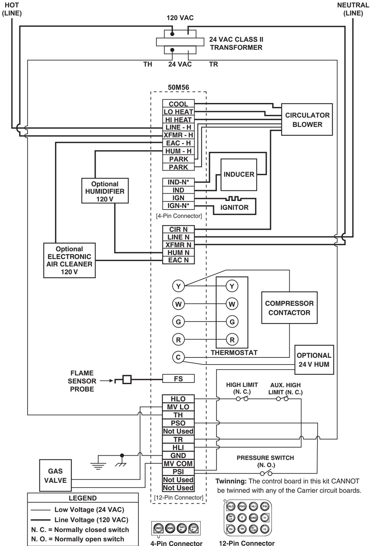
\*Use Line Neutral terminal when replacing new style control.
