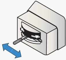
Switch water supply off after use to prevent bursting supply hoses and protect machine solenoid valves.
