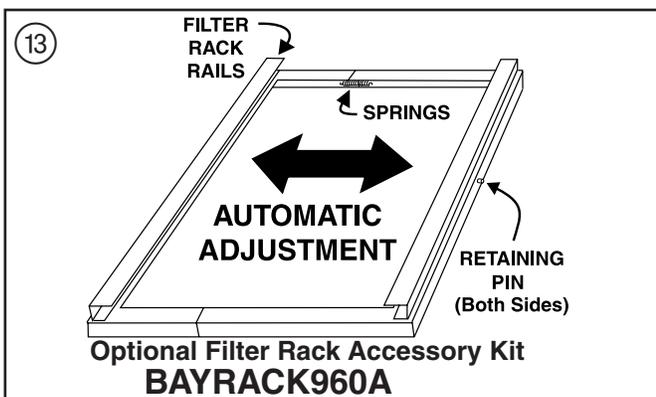
**NOTE:** The narrow 14.5" width furnace cabinet prevents use of the filter rack for right side return. Pre-drill clearance holes and then attach filter clips with the screws provided. The filter clip with the leaf spring mounts in the rear of the cabinet
