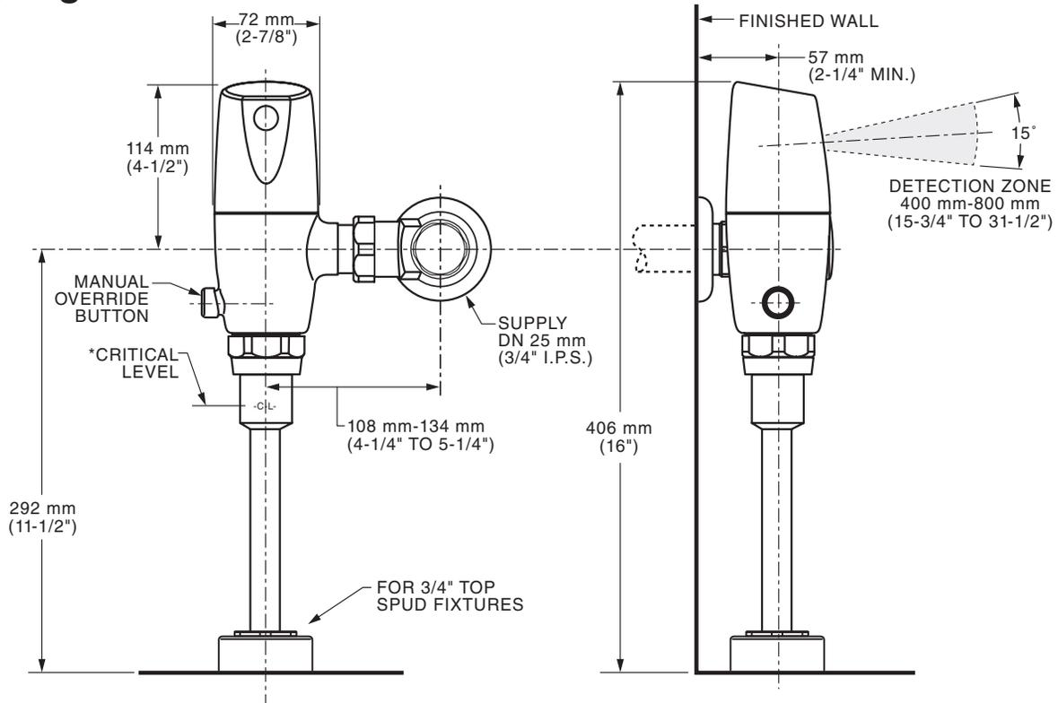
\*Note: The Critical Line (-C-L-) on Vacuum Breaker must typically be 6" (152mm) above fixture. Consult Codes for details.
