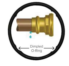
The drip fit O-rings ensure that an unpressed end will drip. This is an added safety feature to ensure unpressed ends are discovered and corrected.
