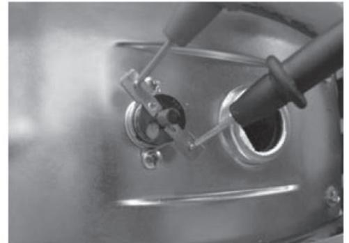
Step 4. If continuity is indicated, the switch is closed, allowing millivolt current to pass.
