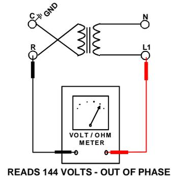
If meter reads approximately 96 volts - the primary to secondary are in phase - if reads approximately 144 volts out of phase - reverse low voltage wires.
