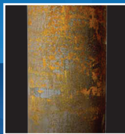
Top Competitor's Glass-lined Tank Very Heavy
