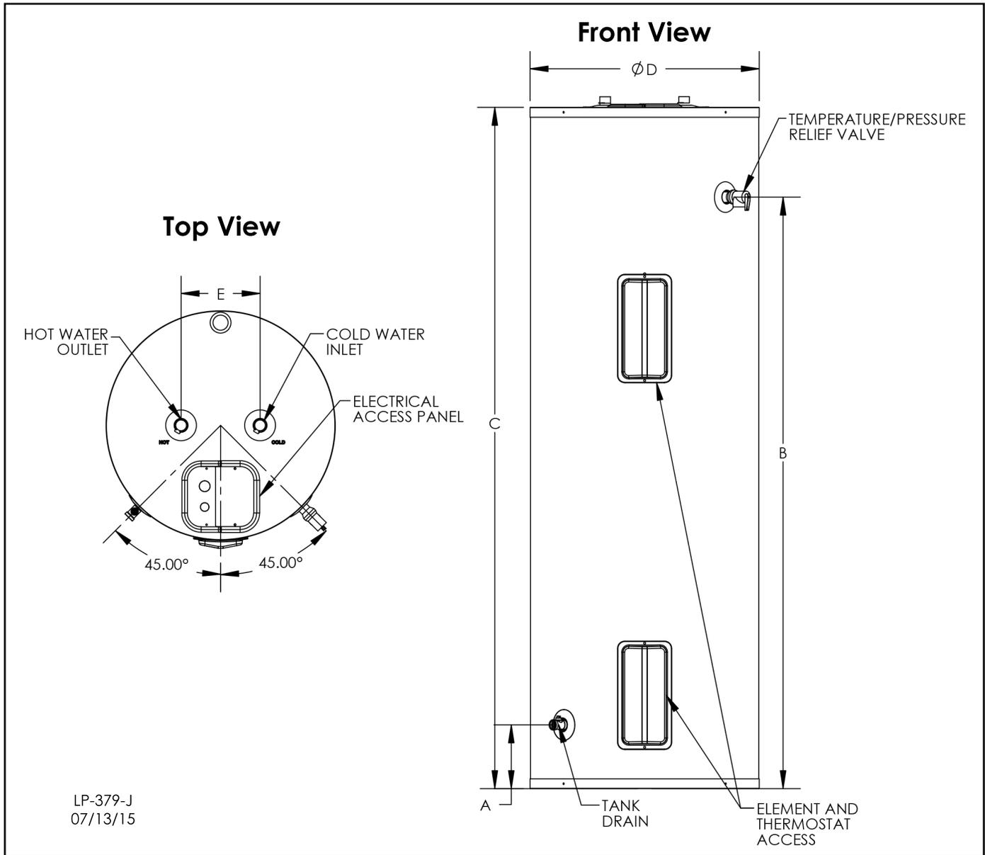
Figure 2 - Dimensional Drawing - Staged Operation
