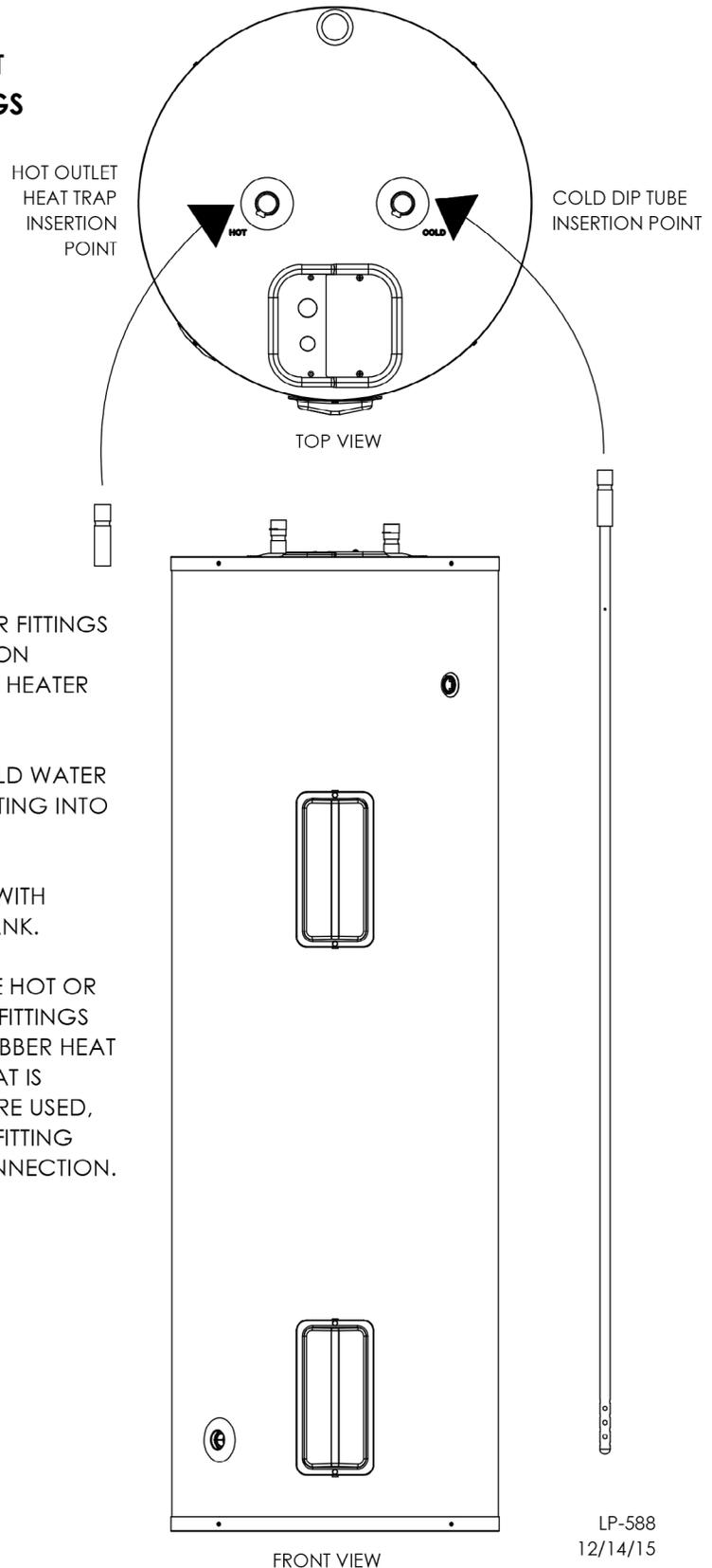
1. THE HOT WATER AND COLD WATER FITTINGS MUST BE INSTALLED IN THE ORIENTATION SHOWN IN THESE DIRECTIONS OR THE HEATER WARRANTY WILL BE VOIDED.
