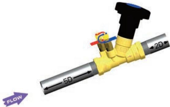
Care should be taken when installing Fig. S1810 (solder end valve) to ensure that the flame is directed away from the center of the valve (valve seat and seals) and also from the P/T ports (seals). This will reduce the risk of damaging the valve seals due to over heating.
