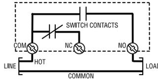
Flow Switch will activate load (alarm, light, relay, motor starter, etc.) when flow occurs.
