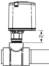
**Do not tighten by grasping the enclosure.** Allow a 1 3/4" space from the bottom of the enclosure to the top of the tee (**Figure 3**) and be sure that the arrow on the side of the enclosure is in the direction of the flow.
