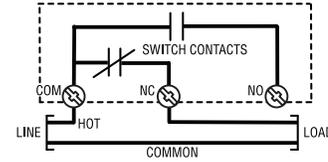
Flow Switch will activate load (alarm, light, relay, motor starter, etc.) when no flow occurs.
