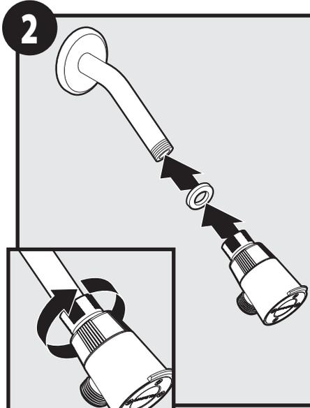
Hand tighten handheld bracket and washer to shower arm.
