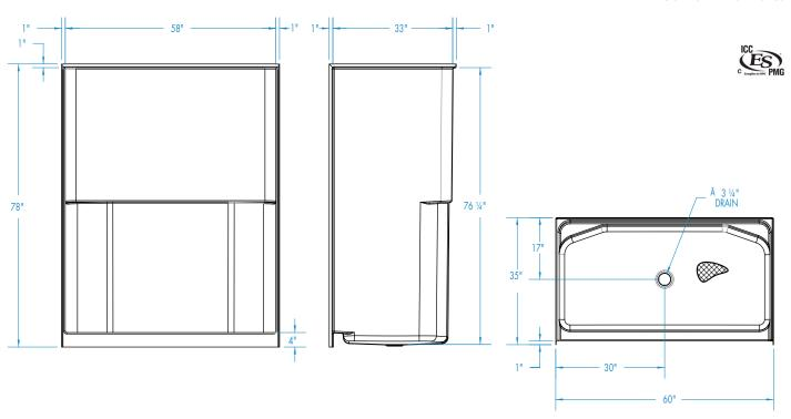
FEATURES lbs Dimensional Tolerance ± %". Dimensions needed for site preparation should be measured from the unit. Aquatic assumes no responsibility for preparatory work.
