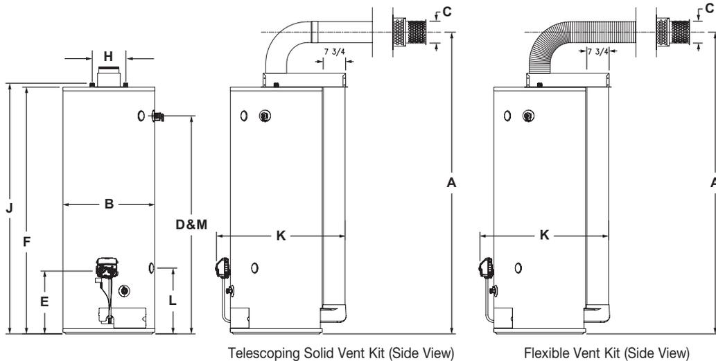
**General:** All gas water heaters are certified at 300 PSI test pressure (2068 kPa) and 150 PSI working pressure (1034 kPa). All potable water connections are 3/4" NPT (19mm). All gas connections 1/2" (13mm).
