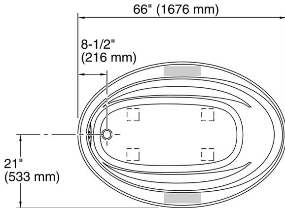
No change in measurements if connected with drain illustrated. (K-37382)
